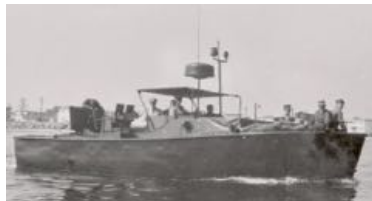
Above: A rare shot of a Mk 4 LCPL conversion by BSU-1 as part of Project ZULU. The LCPL has been fitted with heavy machine guns, gun shields and additional armor. Four LCPLs would be converted and were heavily utilized by MST-2 from 1967 through 1969 when they were replaced by the new MSSC. The problem that plagued both the Project ZULU conversions of the LCM-6 and LCPL Mk 4s were their lack of speed. This was not solved until the advent of the LSSC and MSSC. [Photo: Tom Hawkins]
