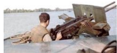
Above: The MST-2 detachment at Vinh Long had an LCPL that had twin .50 machine guns behind a custom armored gun shield. The center plate was designed to stop straight-on shots from hitting the gunner. [Photo: Bill Strawbridge]
