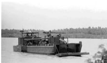
Above: The Can Tho HSSC prior to its last major upgrade in 1969. This last upgrade replaced the Mk 2 Mod 0 81mm mortar (gray
