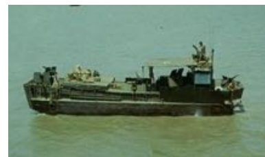
Above and below: The LCM-6 conversion by ST-1 was called the "Mighty Mo" due to its heavy armament. This was the first of the Heavy SEAL Support Craft (HSSC). Two MST-2 purpose-built HSSCs replaced the "Mighty Mo" in mid 1967. [Photos: Jerry
