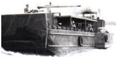
Below: The next major armament upgrade to the Can Tho boat – a GAU-2B/A (M134) 7.62 NATO Mini-gun (rotary barrel machine gun). Note the gun smoke from the Mini-gun that partially obscures the recoilless rifle barrel. [Photo: Bill Moreo]
